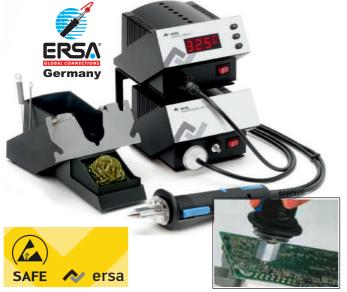
This Desoldering Station is suitable for removing residual solder and for desoldering wired components, even from multi-layer PCBs. The system consists of the Ersa **DIGITAL 2000 A**, a vacuum unit with the **X-TOOL** desoldering iron and the tool holder. The desolderingtip is heated by two PTC heating elements.
