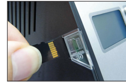
Parameterization thru Micro SD card for of the i-CON Nano
